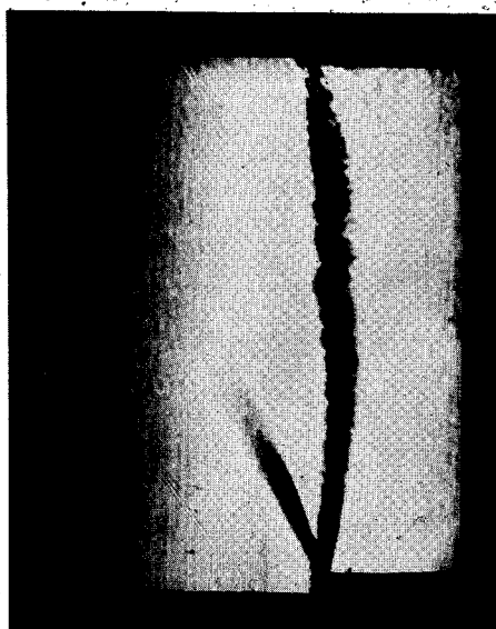
Fig. 2 Schlieren photograph of the shear layer over a notch: L/H = 4 , \lambda = 5.77 in., M_0 = 1.89 .
